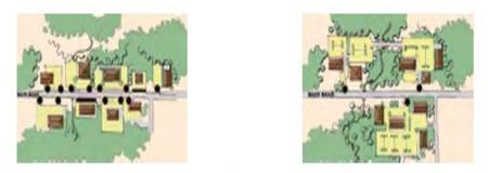
The illustration on the left shows a typical commercial development pattern, the black dots and wide black lines are the entry/exits from the parking areas. The illustration on the right has the same buildings, but through planning for access management and shared parking the road is much safer with far fewer exit/entry points.
