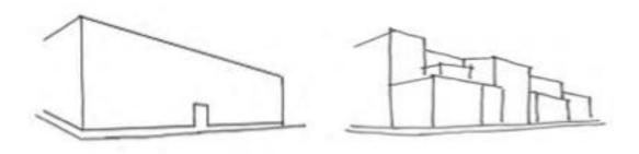
Buildings greater than 20,000 square feet should be designed in a manner to break up their mass into smaller visual components through the use of projections, recesses and varied facade treatments. The two drawings above show how changing the design and massing of a large building can dramatically alter the perceived scale of the building from one large building to many smaller ones.
