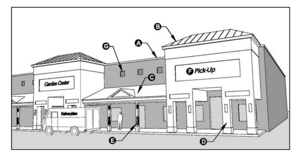
Big-box and other large retail structures are encouraged to articulate their primary façade(s) with various design features to help reduce the overall scale of the building. The use of roofline articulation or mass divisions is encouraged and can be used to highlight entry points, exits, specialty areas (such as a garden or landscaping center, auto service, customer pick-up zones, or separate places of business.
